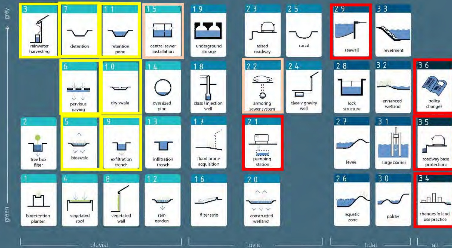
Figure 171. “Periodic table” menu of green and grey infrastructure technology options. The menu is organized to address various flooding types, from pluvial (rainfall and runoff mitigation in upland areas), fluvial (runoff, high groundwater, and surface water management in low-lying flood-prone areas), tidal (flooding associated with storm surge, high groundwater, and tidally influenced), and all (applies across the spectrum).
