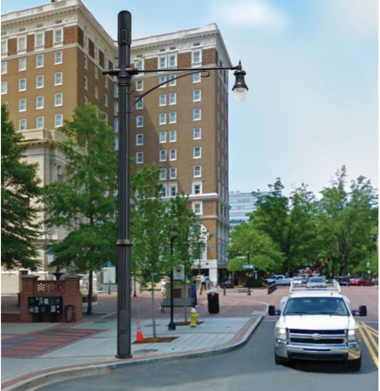
Exhibit 1. Simulated fluted pole to be manufactured by Nepsa with capacity for two internal, collocated wireless antennas. Decorative mast arm and down lighting luminaire by Sternberg Lighting. This would may be an acceptable design, depending on the location context; however, the pole’s location, mere inches from the curb, would violate the 8 foot clear space requirement from the curb or edge of pavement.
